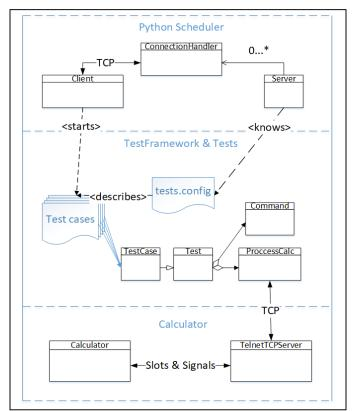
Fig. 2. Architecture of the proposed system for parallel software product testing
